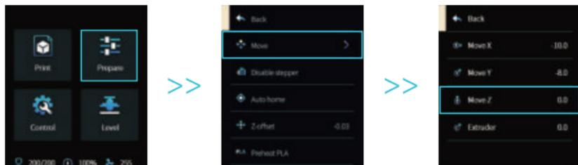
4. Enter "Prepare → Z-offset", adjust the Z-axis compensation value so that the height from the nozzle to the platform is almost the thickness of A4 paper (0.08–0.1mm), click the knob to confirm, and complete the center point leveling.
